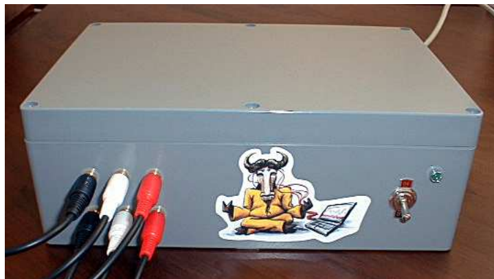
Figure 3.7: The completed ModularEEG device
