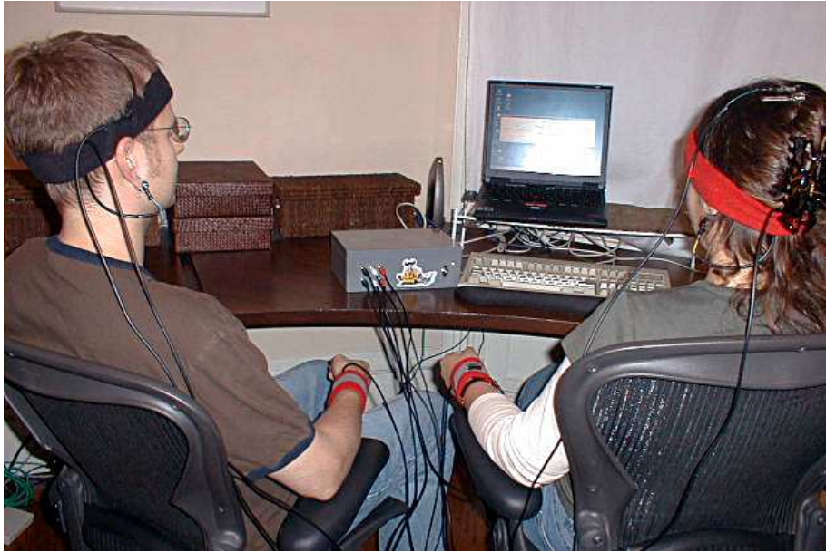
Figure 3.2: Two Brainathlon players connected to the ModularEEG device
